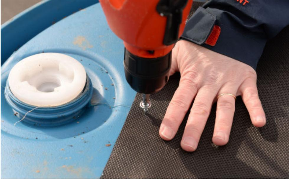
Attach the fabric cloth with 8 self-tapping screws. The fabric will help keep organic matter and critters out of your barrel.
