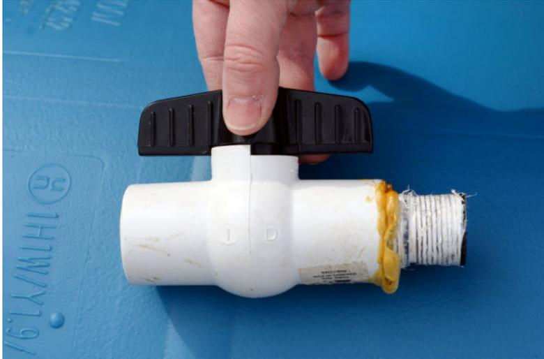
Use a PVC (shown) or brass at the bottom of the barrel, apply plumbers tape to help prevent leaks. Attach about six inches from the bottom to allow easy attachment of the hose and allow sediment to settle to the bottom.
