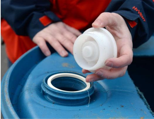
Use bung plugs, found at a plumbing supply store, to close up the bung holes. This allows for easy access to the inside.
