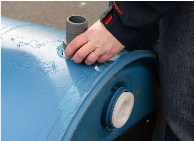
A hole saw is used to drill an opening near the top for the overflow drain. Barrels can also be fitted together at this juncture if more than one is desired.
