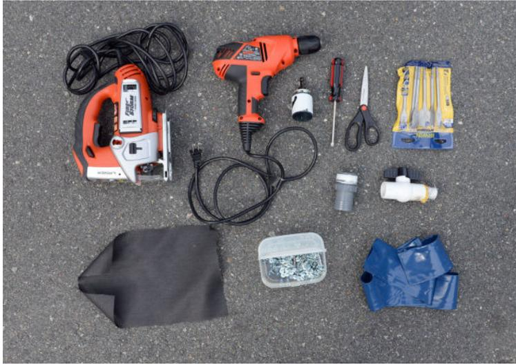
Tools you will need include, clockwise from top left, a jigsaw and blade, 3/8" drill, hole saw bit, Phillips screwdriver, scissors, spade blade drill bits, treaded PVC pipe fittings and valve, lay flat discharge hose, self tapping screws, garden fabric. Not pictured are food grade barrell and bung plugs.
