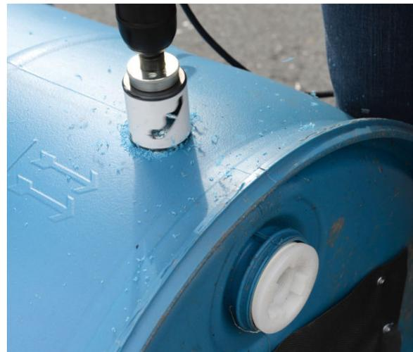
A hole saw is used to drill an opening near the top for the overflow drain. Barrels can also be fitted together at this juncture if more than one is desired.
